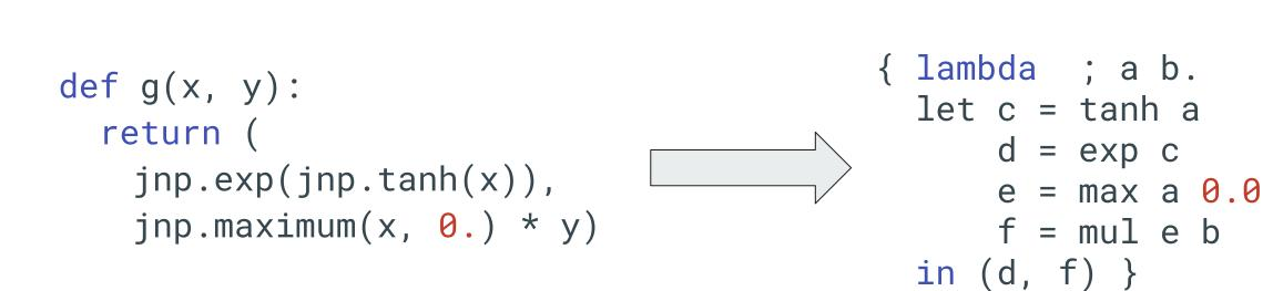
JAXPRs are composed of JAX *primitives*, or the lowest level traceable operations in JAX.
